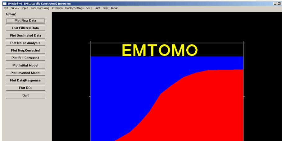
The program needs you select the equipment used for acquisition. Go to Input and Input Sensor and choose the PROFILER. After click OK.
