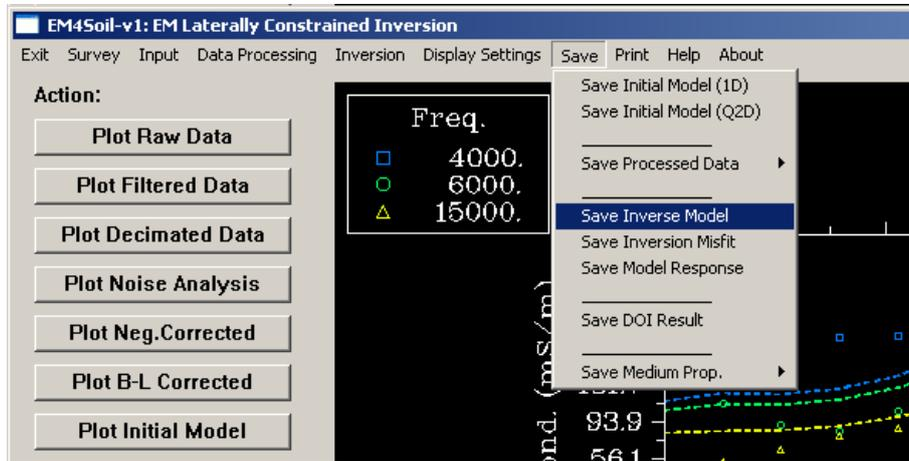
**NOTE:** if your data have negative values (even if they have been corrected) the program does not do an initial model. In such case before the inversion you must define an initial model. Go to Inversion, define initial model (see the sequence of screens):
