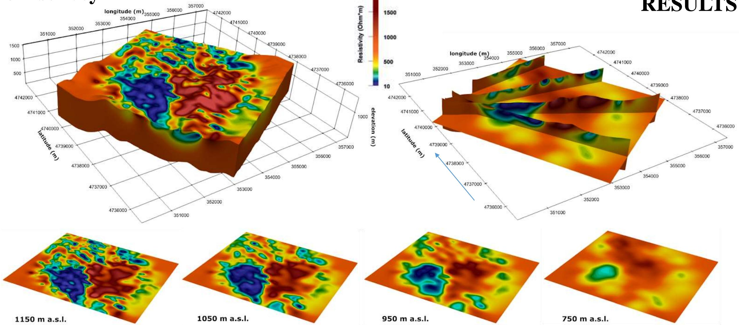
**Top left:** 3-D Fullwaver resistivity model of the entire survey area. **Top right:** 2-D cross-sections over the horizontal slice at 750 m a.s.l. **Bottom:** slices at different absolute elevations. The wide low-resistive region delineates the deeper portion of the PGC basin infill. Those slices suggest a complex structure with a main depocenter to the south and segmentation to the north, due to the interference of differently oriented fault systems
