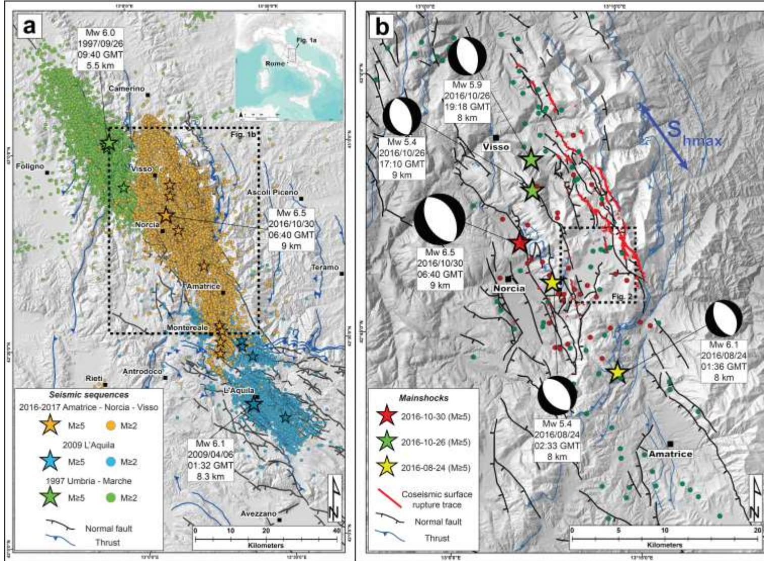
a) Quaternary normal faults (black lines), principal thrusts (blue lines) and the three main seismic sequences occurring since 1997 (the stars indicate events with  $M>5$ ). b) Sibillini Mts. area, showing the trace of the coseismic surface ruptures following the 30 October 2016 Mw 6.5 Norcia earthquake (modified after Civico et al., 2018) and focal mechanisms of the mainshocks of the Amatrice-Visso-Norcia sequence.
