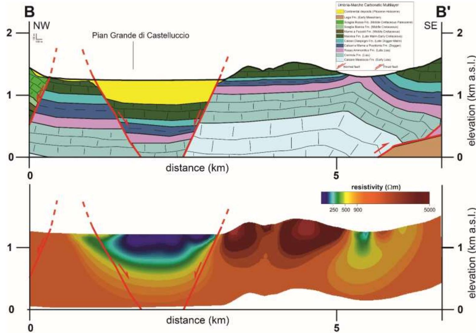
Sketch of **possible deep fault networks** as inferred from the recovered 3D resistivity model (elevation slice at 900 m a.s.l.).
