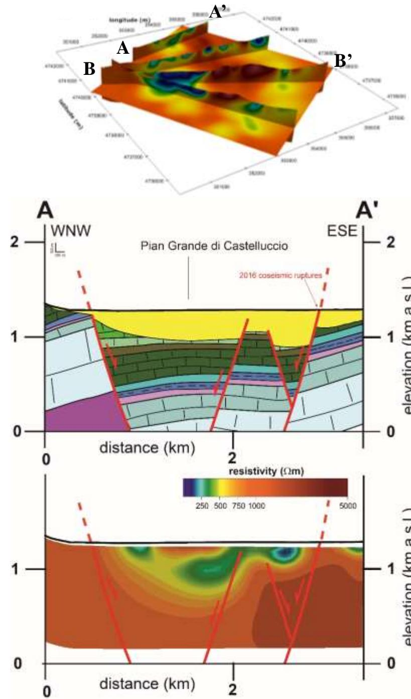
Two simplified geological cross-sections in the northern (A-A') and the southern part of the basin (B-B') – see left panel for the location of the interpreted sections
