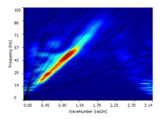
If the source was at the other end of the geophones line, spectrum obtained was similar to that shown in the figure. In this case the line on which the energy is indicative of a apparently negative propagation speed.
