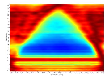
SWAN makes visible the spectrum on the REMI method normalizing it for every frequency to increase the graphic contrast with the background noise even at frequencies where micro-tremors are weak.
