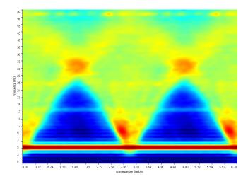
By observing the symmetry of the spectrum in the central area, or at the junction between the two copies of the spectrum, there can be an indication of how satisfied the hypothesis of isotropic sources is. In this case, neglecting a slight asymmetry quite evident around the frequency of 10 Hz, the spectrum is symmetrical enough to be able to proceed with processing.
