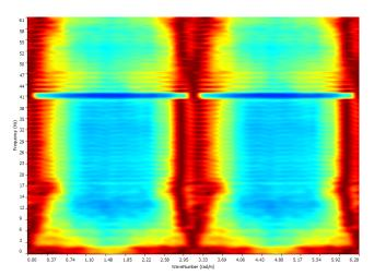
During the interpretation of spectrum task, the objective is to estimate the actual speed of propagation of the seismic wave at different frequencies. The experimental dispersion curve is nothing but all of these obtained speeds in the frequency range of interest.
