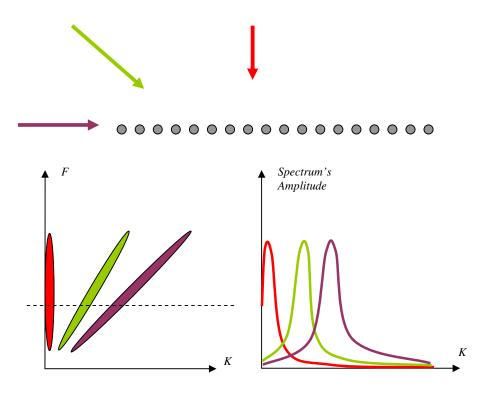
In typical FK spectrum (REMI) you will see the overlap of the effects of various micro-tremors. This overlap is shown in the figure, where you can see the composition of a simulated section (at a given frequency) FK spectrum since the effects of individual microt-remors. The dashed vertical line is an indication of the actual speed at this frequency. As it can be seen, there are overlapping effects associated with apparent speeds of greater value (or associated with a wave number lower K).
