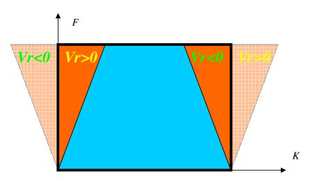
In figure, finally showed a spectrum FK on the REMI method. It is noted that the area coloured in red, indicating the presence of energy, can be reduced to speed apparent positive and negative. You notice any apparent speed also very high in absolute value. There is also a lack of energy (area coloured in blue) at speeds below a certain threshold, confirming the expectations. This threshold is, as shown above, linked to the actual speed of propagation in the soil in the wave analysis.
