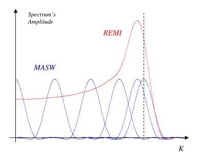
Shown in the figure is a real example of FK spectrum for MASW data.
