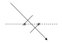
As the angle between the path of the wave and the geophones axis increases, also increases the apparent speed calculated. The limit situation is when the direction of propagation is perpendicular to the axis: in this case the apparent velocity measured will be very high (infinite). This is because the time lag observed between the two geophones will be virtually nil.
