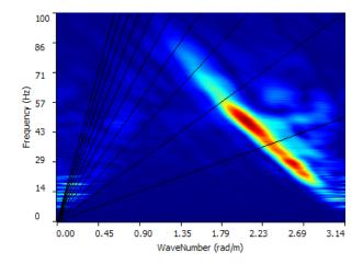
To facilitate the interpretation of this spectrum we should take into account the cyclicality of the spectrum as a result of the properties of the Fourier transform.
